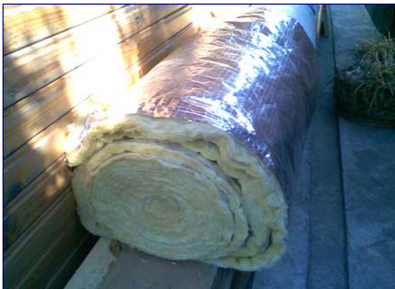
Photo 13 The glass wools used for isolation (source, http://www.douamaini.ro/ )
